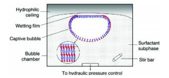
Fig. 8: Schematic diagram of a CBS. The captive bubble floats against the hydrophilic ceiling but is separated from it by a thin wetting film. The inset shows multilayer structures of the adsorbed PS at the air-water interface of the bubble. The surface tension is determined by bubble shape analysis. Surface area manipulations are conducted by altering the hydraulic pressure in the chamber (reproduced from [Zuo *et al.*, 2008] with permission from the Elsevier)
