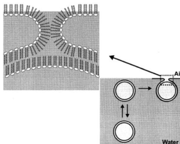
Fig. 9: Enlarged view of final step of adsorption; transfer of surfactant in the air–liquid interface (reproduced from [Schram and Hall, 2001] with permission from the Elsevier)
