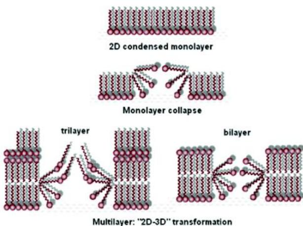
Fig. 11: Schematic diagram of film collapse
