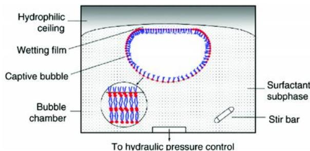
Fig. 8: Schematic diagram of a CBS. The captive bubble floats against the hydrophilic ceiling but is separated from it by a thin wetting film. The inset shows multilayer structures of the adsorbed PS at the air–water interface of the bubble. The surface tension is determined by bubble shape analysis. Surface area manipulations are conducted by altering the hydraulic pressure in the chamber (reproduced from [Zuo *et al.*, 2008] with permission from the Elsevier)
