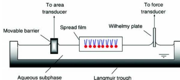
**Fig. 6: Schematic of a Langmuir-Wilhelmy balance (LWB).** The surfactant film is usually formed by spreading at the air-water interface of the aqueous subphase filling the Langmuir trough. Moving the barrier to the right decreases the area of the spread film, thereby increasing surface pressure (www.wn.com)
